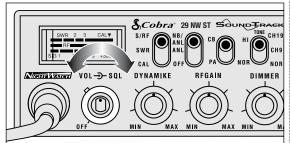
To achieve the Desired Squelch Setting (DSS), turn the Squelch control ⊚ counterclockwise until you hear noise. Now turn the control clockwise just until the noise stops. This is the DSS setting.
